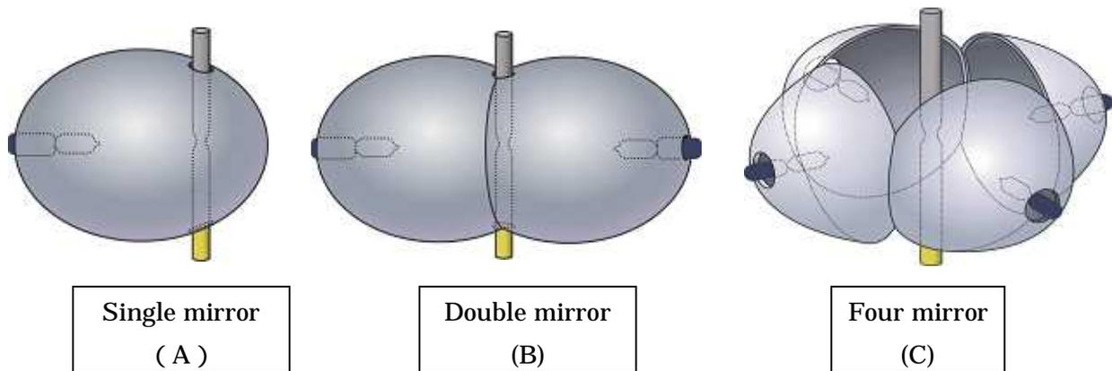
**Fig.1** Three types of the focusing system for the optical floating zone furnace.
