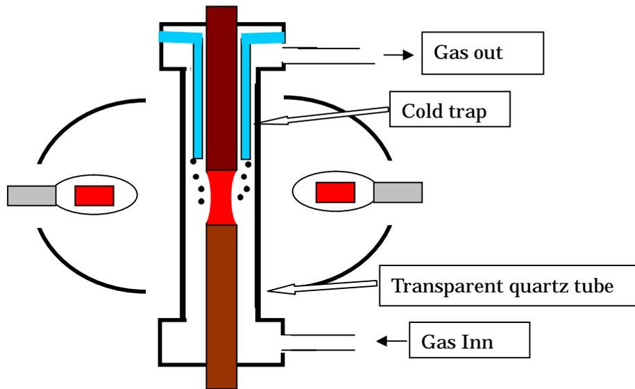
Fig.4 Schematic diagram of the cold trap inserted in the quartz tube and focusing scheme. Small particles from the molten zone would be condensed on the cold trap rather than the surface of the quartz tube, then can keep its clean condition more long time compared to the normal case without the cold trap.
