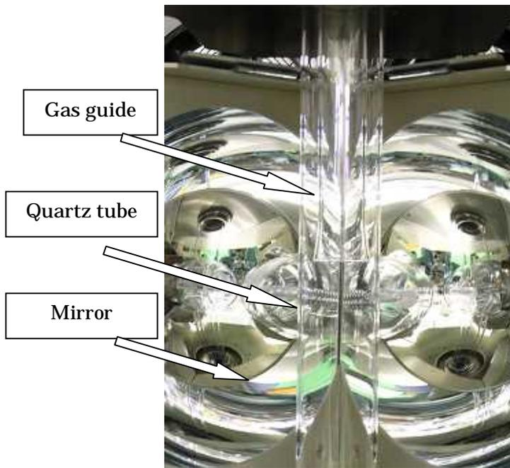
Fig.7 Feature of the gas guide inside the quartz tube
