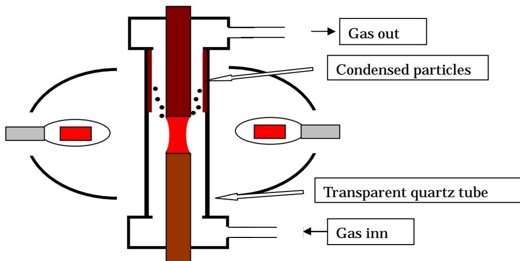
Fig.3 . Schematic illustration of the optical floating zone furnace.
