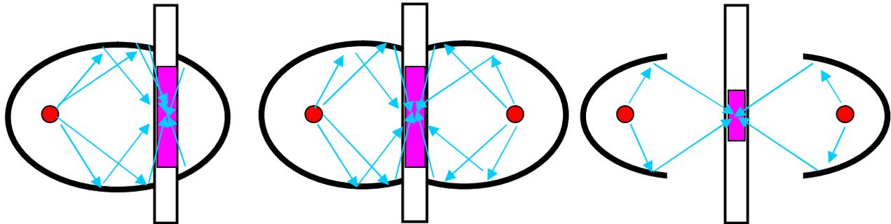
Fig.2 The Effective zone for the focusing of the infra red rays in the corresponding different mirror systems. The length of this zone in the four mirror furnace is much shorter than that of both the single and the double mirror system.
